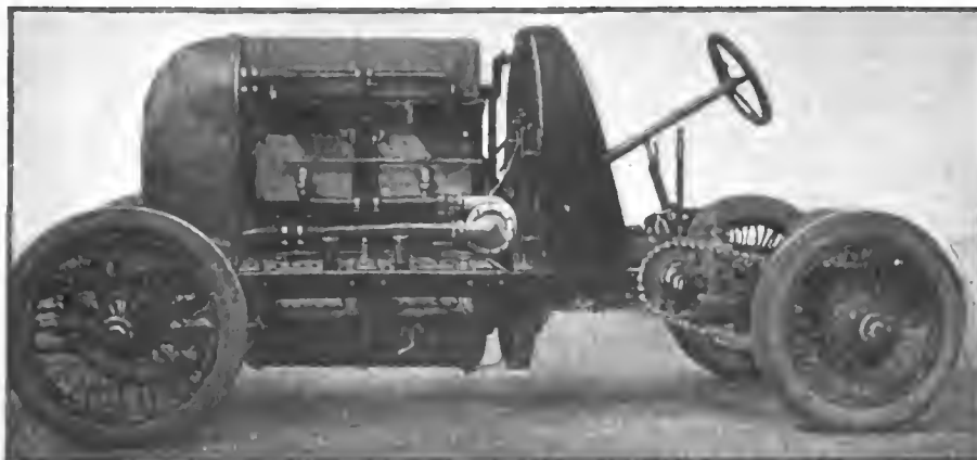
Exhaust side of 300-hp. Fiat chassis. This view gives an idea of the height of the motor in proportion to the wheelbase
